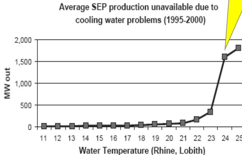
Fig. 2. Average production unavailable due to cooling water problems before deregulation.
